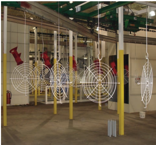
Grain Systems International powder coats components used on its line of grain storage and drying equipment.
