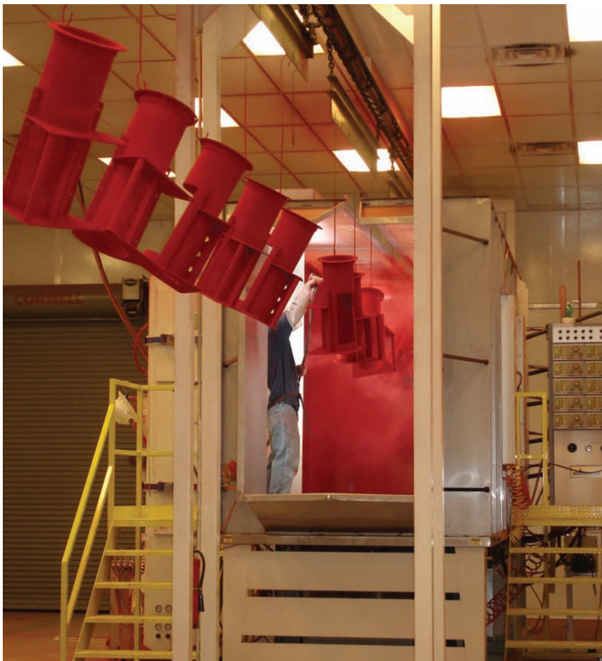
Two powder coating booths housed in an environmental room apply powder by using a combination of automatic and manual equipment.
