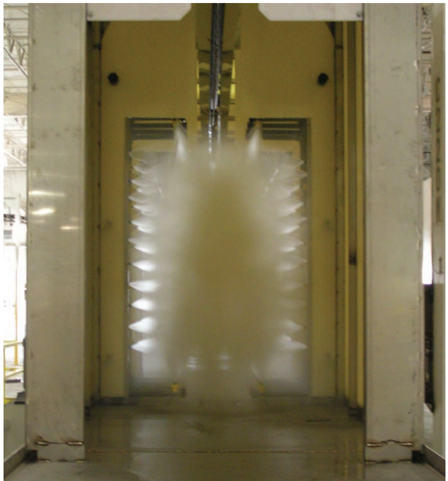
Galvanized steel components pass through a three-stage washer consisting of an iron phosphate, rinse, and seal rinse.
