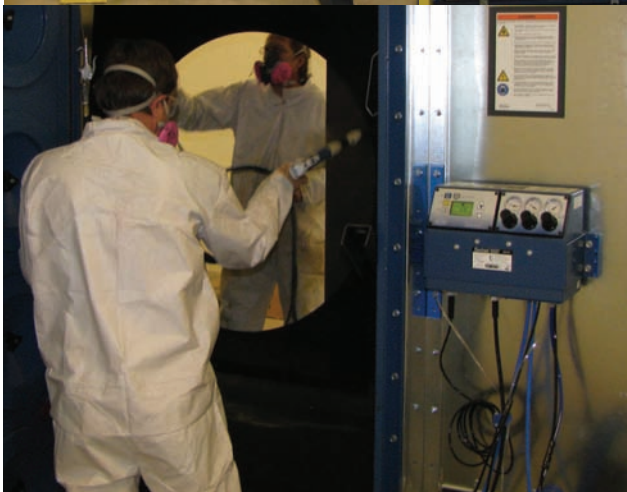
Two spray operators manually apply powder inside the system’s environmental room.
